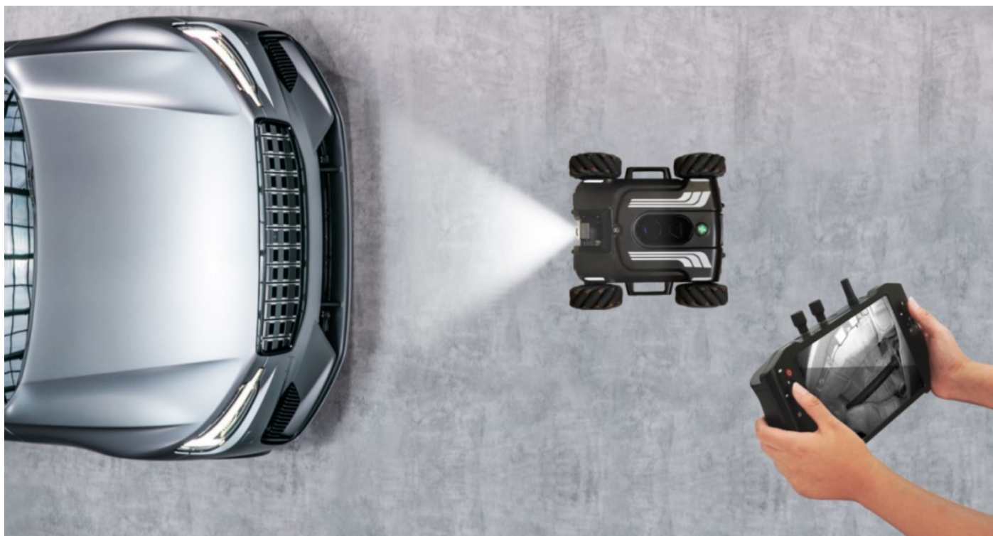
CDC-100 Vehicle chassis inspection robot (vertical view picture)
